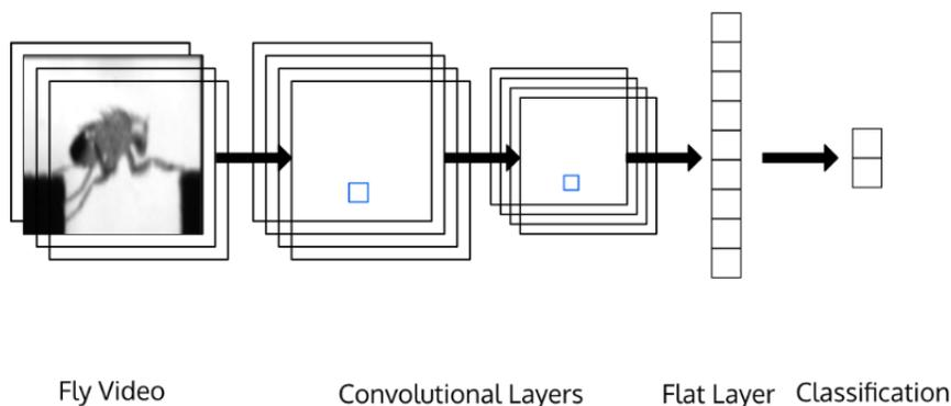
Figure 3: Convolutional Neural Network Model Example. My project uses 3D convolutions to process the data.
